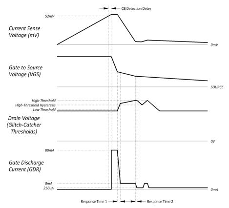
Figure 9 - Circuit Breaker (CB) and Glitch-Catcher<sup>™</sup> waveforms.
