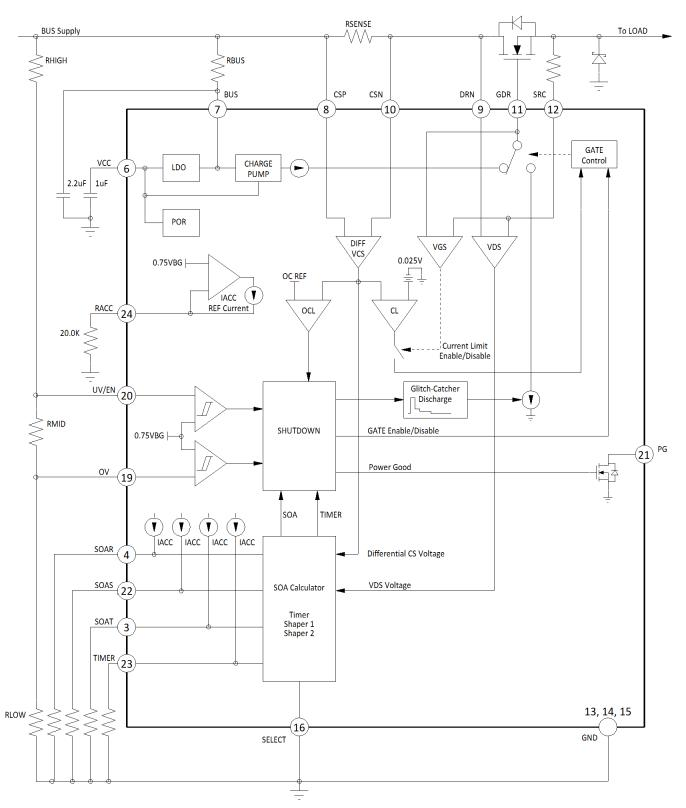
Figure 12 - PI2211 Block Diagram.
