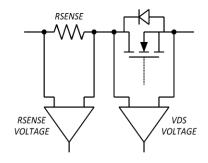
Figure 15 - MOSFET Power measurements.
