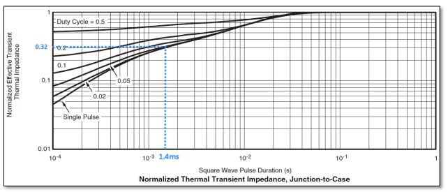
*Figure 16 - Determining the pulse width.*
