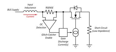
*Figure 8* - *Glitch-Catcher™ Over-current fault detection circuit.*
