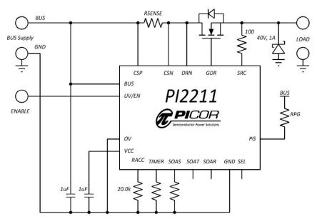
Figure 1 – Typical PI2211 application schematic.
